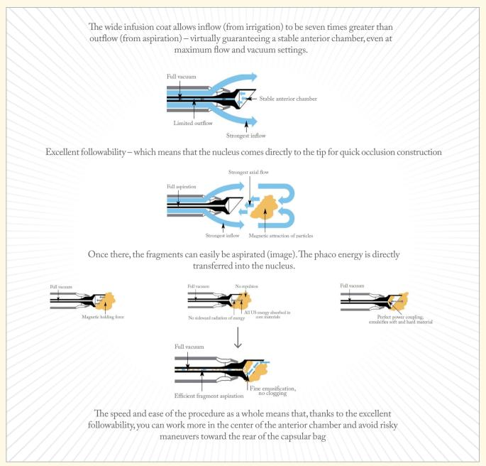
Figure 3. easyTip® and benefits of using high vacuum and flow settings.
