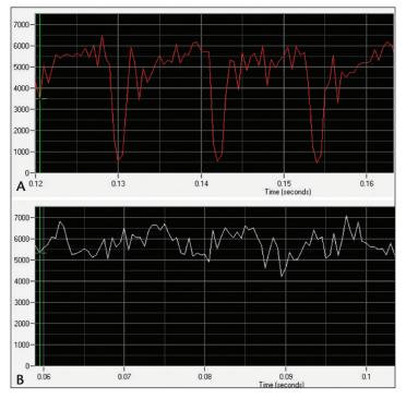
Figure 4. Graphs depicting flow rates in traditional guillotine-style cutters (A) and the Continuous Flow-Cutter with the OS4 platform (B). Whereas the flow is intermittently interrupted by the closed action of the blade in graph A (identified as zeroing of the flow), the flow is relatively stable in graph B.
