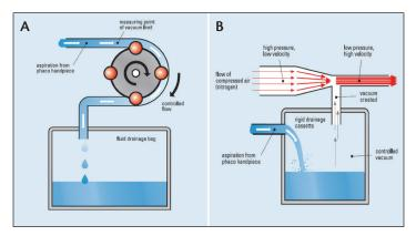
Figure 2. Peristaltic pumps (A) employ rollers to compress the tubing system to create flow while a preset vacuum level is engaged when the port is occluded. As the port becomes occluded, the rollers slow down, yielding decreased outflow. Venturi systems (B) operate on a different principle, where the flow is generated by compressed air, the air nozzle is connected to a closed drainage bag, and vacuum is constantly on.
