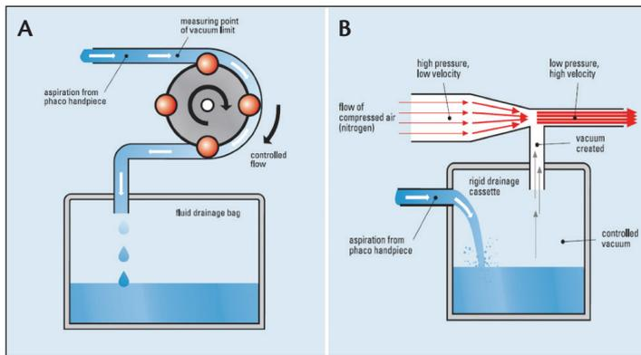
**Figure 2.** Peristaltic pumps (A) employ rollers to compress the tubing system to create flow while a preset vacuum level is engaged when the port is occluded. As the port becomes occluded, the rollers slow down, yielding decreased outflow. Venturi systems (B) operate on a different principle, where the flow is generated by compressed air, the air nozzle is connected to a closed drainage bag, and vacuum is constantly on.
